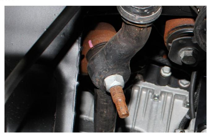
4) Unscrew the large nut holding the pitman arm to the steering box using a 46mm open end wrench, or an 18" adjustable wrench.
