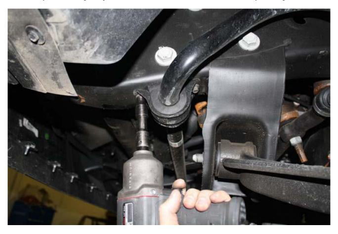
3) Unscrew the factory lock nuts that hold the drag link to the pitman and idler arms, using a 24mm deep socket, and discard them.
