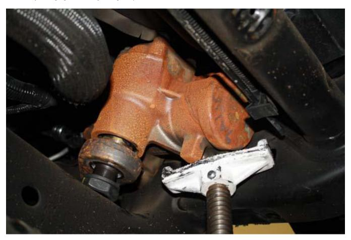
7) Loosen the nut holding the idler arm to the idler arm pivot with a 30mm end wrench. Then unbolt the idler pivot from the frame and pry it out of the mounting pocket.
