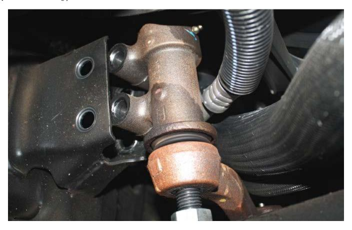
8) There are 2 pitman arm support brackets included in this kit, as of June 20th, 2011. On some of the 2011 and newer GM trucks, there is a new design center link that has a large rubber bushing in the center link where the pitman arm attaches to it. If this vehicle has the new center link, you must use pitman support bracket #3002. If this vehicle has the traditionally designed center link, use the pitman arm support bracket #3001.
