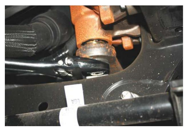
5) Unbolt the steering box from the frame by removing the 3 bolts using a 21mm socket.
