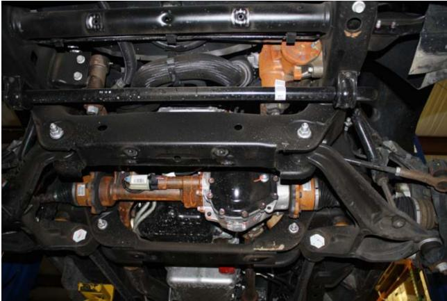
2) Unbolt the sway bar mounting clamps from the frame with 10mm socket and let the sway bar hang from the end links.
