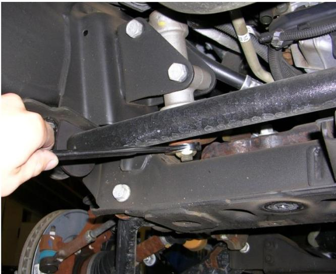
5) Apply a small amount of thread locker on all of the threads on both of the 5/8"x 3/4" rod ends, then thread one 5/8" jam nut all the way on to both of the rod ends as shown in Figure 1. Then insert the rod end through the 5/8" diameter hole on both the pitman and idler arm brackets as shown below. Now thread a second jam nut on to both rod ends, but do not tighten at this time.
