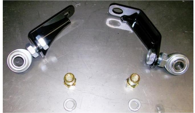
6) Insert one lock washer over each of the drag link studs, and then install the pitman and idler arm brackets on to the pivot ends where hardware was previously removed in steps 3 and 4, at the same time place the rod end which is connected to the Full Throttle Suspension brackets over the drag link studs so that the lock washer is in between the Full Throttle rod end and the drag link.
