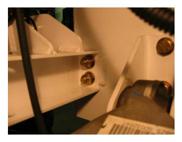
41) Reinstall sway bar end links connecting lower control arms to sway bar on both sides of vehicle, and tighten the link hardware to factory spec. CAUTION: do not over-tighten sway bar links; the bushings do not need to "squeeze out" the sides, this is a common misconception.
