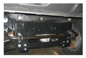
40) Position lower control arms into drop brackets using two  $5/8 \ge 5''$  and two  $5/8 \ge 6''$  bolts and nuts, DO NOT TIGHTEN at this time.
