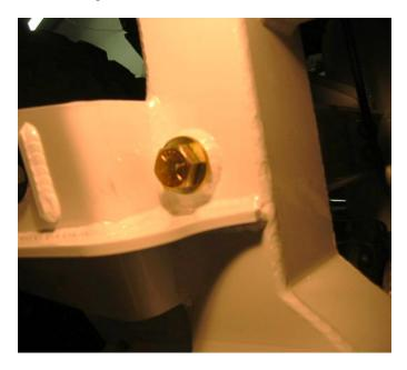
25) Install the factory bump stops into the holes on both sides of the rear lower control arm cross member
