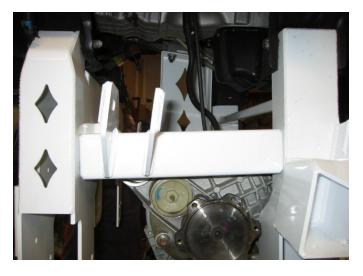
24) Install the upper a arm drop bracket to the rear cross member using the  $5/8 \ge 6$ " bolts and hardware.
