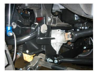
56)Center up the eccentric alignment washers within the range of the upper control arm drop brackets, then tighten the nuts as shown. NOTE: the alignment shop will likely change the position after final assembly, this is just a preliminary setting.
