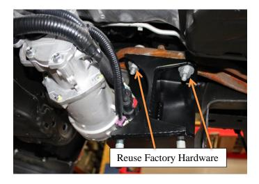
2) Locate 8512 Driver side Differential brackets and the factory diff hardware. Install the brackets to the factory mounts with the taller part of the brackets to the front of the truck with the factory hardware.
