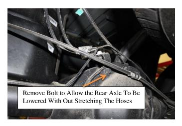
3) Remove the ABS line clip from the top of the frame and at the axle.
