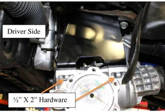
4) Re-connect the electrical and vacuum connections back onto the differential.
