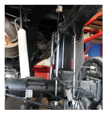
10) Locate 8512 Brake Line Bracket and the supplied 5/16" hardware. Attach the new bracket to the differential and attach the brake line to the new bracket. Torque to 20 ft lbs.
