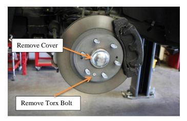
6) Remove axle nut cover, axle nut, washer, and rotor with hub bearing. Retain hardware for reinstallation.
