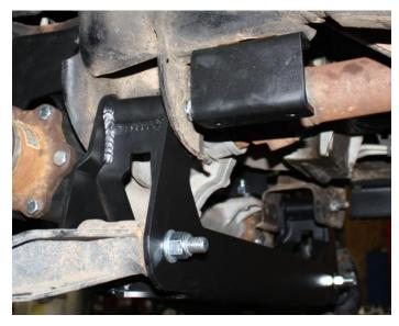
24) Mark the lower control arm. drill a 11/16" hole 2" over from the stock hole as shown below.
