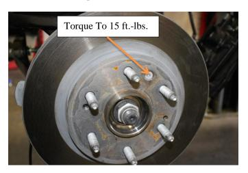
19) Install brake caliper using factory hardware.
