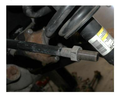
22) Screw the outer tie rod onto the inner tie. Then attach tie rod end to the knuckle with the factory hardware. torque to 45 lbs.
