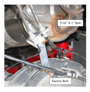
11) On the driver's side, insert the previously removed upper ABS line clamp into the existing hole on the inside of the frame. Re-insert the lower ABS line clamp back into the stock location. Use zip ties and attach the ABS line to the U-Bolt. Keep the line taught at the block and ensure that there is enough slack in the line for full travel of the rear axle.
