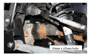
14) Locate the steering knuckle 8400R & 8400L. Attach the lower control arm to the knuckle using the stock hardware and torque to 70 ft.-lbs. Attach the upper control arm to the new knuckle using the factory hardware and torque to 35 ft.-lbs. as shown in picture below.
