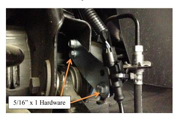
29) Re-route the brake hose and the ABS Line to the steering knuckle using a zip tie to the back of the steering knuckle. Route the ABS line next to the brake hose. Re-connect the ABS line to the harness in the wheel well. Using zip ties secure line to the hose and away from the tire and wheel.
