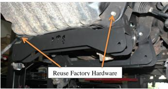
10) Install the lower control arm using the 5/8" x 5" threw the front cross member and the 5/8" x 6" threw the rear cross member.
