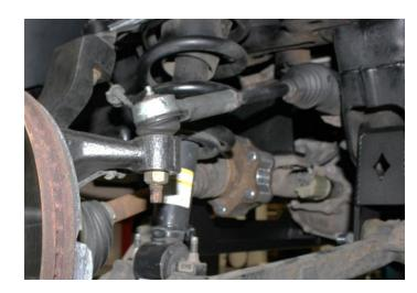
23) Locate 8404 Sway Bar Frame Bracket, and four 10mm stock CV axle bolts with supplies washers. Position the frame bracket on the frame so that sway bar will be farther back from the suspension and attach with the 10mm hardware.
