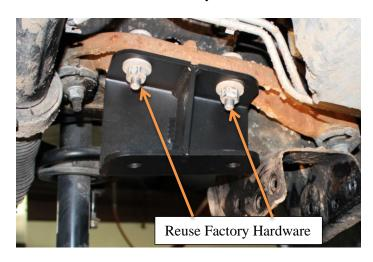
2) Locate 8402 Driver side Differential brackets and the factory diff hardware. Install the brackets to the factory mounts with the taller part of the brackets to the front of the truck with the factory hardware.
