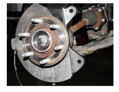
18) Install brake rotor on to factory hub assembly, Install Torx screw and torque to 150 ft.- lbs.
