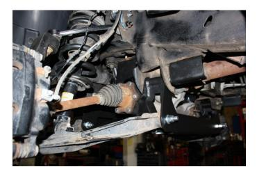
28) Locate 8511 Brake Line Bracket and 5/16"x 1" hardware. Position the new bracket into the factory brake line bracket location and attach with the factory hardware and the 5/16" hardware. Attach the factory brake line bracket to the new bracket. **Carefully** bend the hard brake line and attach with the supplied 5/16" hardware. Torque to 15 ft.-lbs. As shown in picture below.
