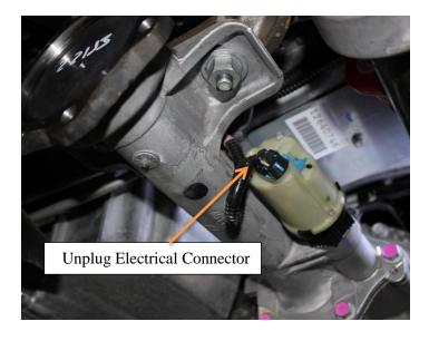
17) Remove differential housing assembly from vehicle. Retain hardware for reinstallation.
