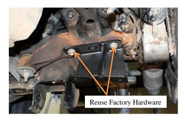
3) Using the supplied ½"x 2" & 5/8"x 2" hardware. Install the diff onto the new drop brackets using ½" hardware on the driver side & 5/8" on the passenger side as shown in picture below. Torque the stock & ½" hardware to 75 ft. lbs & the 5/8" to 95 ft.-lbs.
