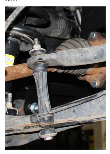
27) Then Torque the 5/8 lower control arm bolts to 110 ft lbs.
