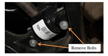
12) Remove the lower control arms from the frame and retain with the hardware for reinstallation.
