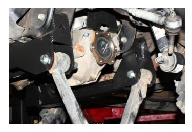
11) Using the stock hardware connect strut to lower control arms and tighten.
