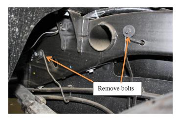
5) Remove the rear shocks and discard, Retain hardware for reinstallation.
