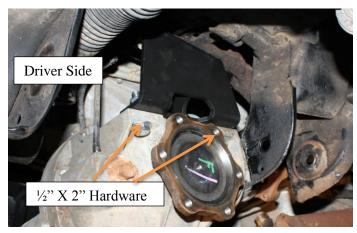
4) Re-connect the electrical and vacuum connections back onto the differential.
