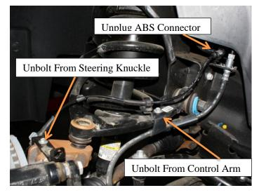
4) Remove the caliper from the steering knuckle and secure the brake caliper to the frame out of the way.
