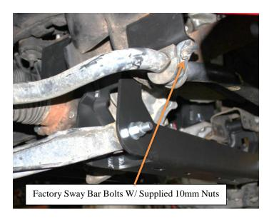
26) Locate the factory sway bar end links and attach to the mount and the lower control arm. As shown in picture below.
