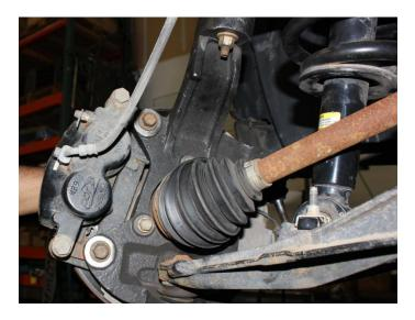
20) Remove the factory outer tie rods, leaving the factory jam nut on the inner tie rod. Cut 3/8" off the outer tie rod.
