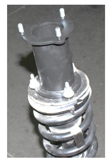
8) Reinstall the struts back into the vehicle using the supplied 7/16" Nylock and washers.
