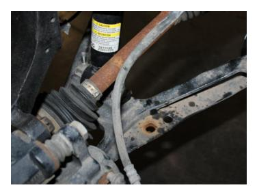
25) Locate the factory sway bar with the factory mounts and attach to the new brackets using the Stock bolts and supplied nuts and torque to 35ft.-lbs. as shown in picture below.
