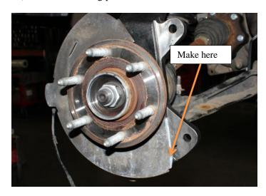
17) Using a die grinder, trim the backing plate as shown below
