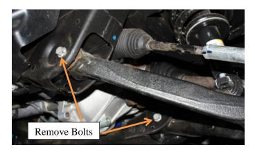
13) Disconnect and Remove CV axles from differential housing.
