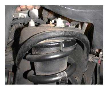
7) Install the strut spacer on top of the factory strut using the factory hardware.
