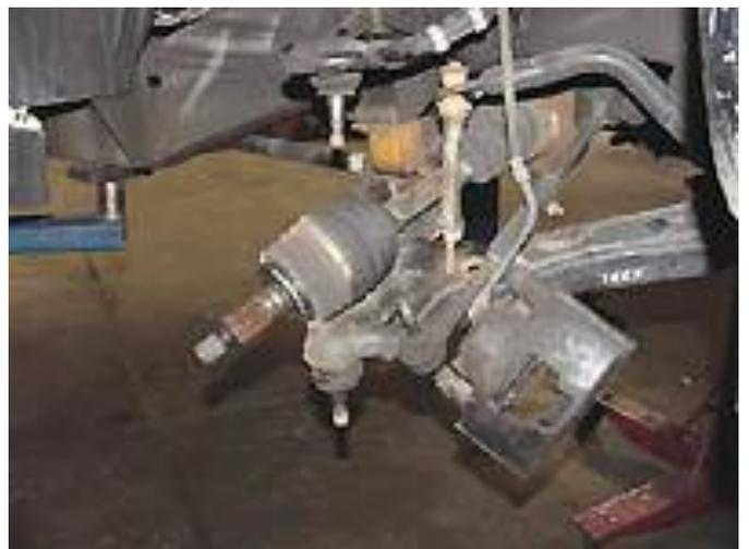
9) Remove cotter keys and loosen the nuts attaching the upper and lower ball joint studs to the knuckle. Separate the ball joint studs from upper and lower points of the knuckle using ball joint (pickle fork) separator, or by striking the knuckle directly adjacent to the ball joint stud with a ball peen hammer. NOTE: Leave both upper
