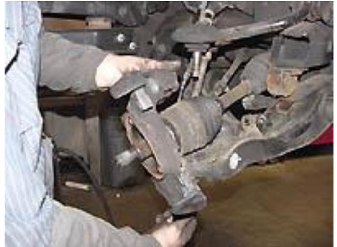
8) Remove nut from bottom of sway bar link on each side.
