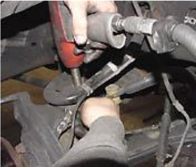
4) Remove brake calipers and hang up out of the way with tie wire to the vehicle frame or bumper brackets. DO NOT let calipers hang by brake hoses. Remove brake rotors and label them for left and right side of vehicle.
