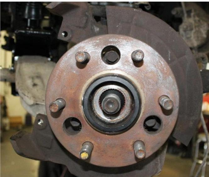
41) Install the brake rotor ,caliper and tie rod as shown, tighten to factory specs.
