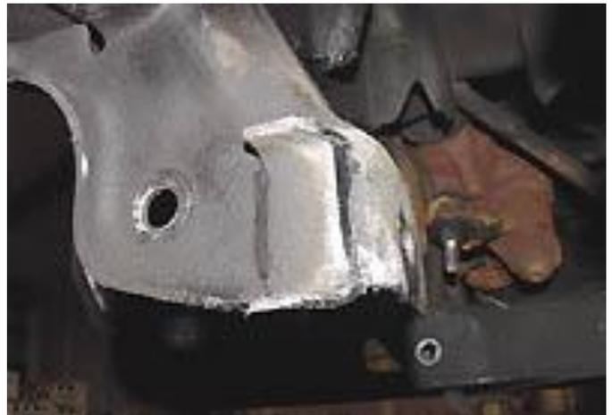
21) Next cut and remove the factory bump stops FLUSH with frame rail, or at least flush with the outer face of the shock tower as shown.
