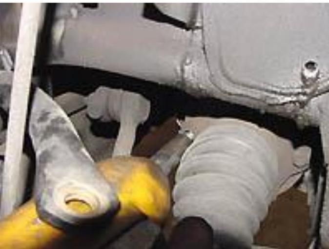
13) Remove two lower control arm pivot bolts and carefully remove and set aside torsion bar and lower control arm (it will be heavy). Repeat these steps on opposite side of the vehicle.
