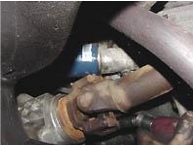
17) Unplug and unclip the 4x4 switch and actuator wires from the right side axle tube and hang them out of the way. Unplug the rubber vent hose from the left side of the differential third member assembly. Remove the two nuts and bolts holding the right side of the differential assembly to the channel shaped right side mounting bracket.
