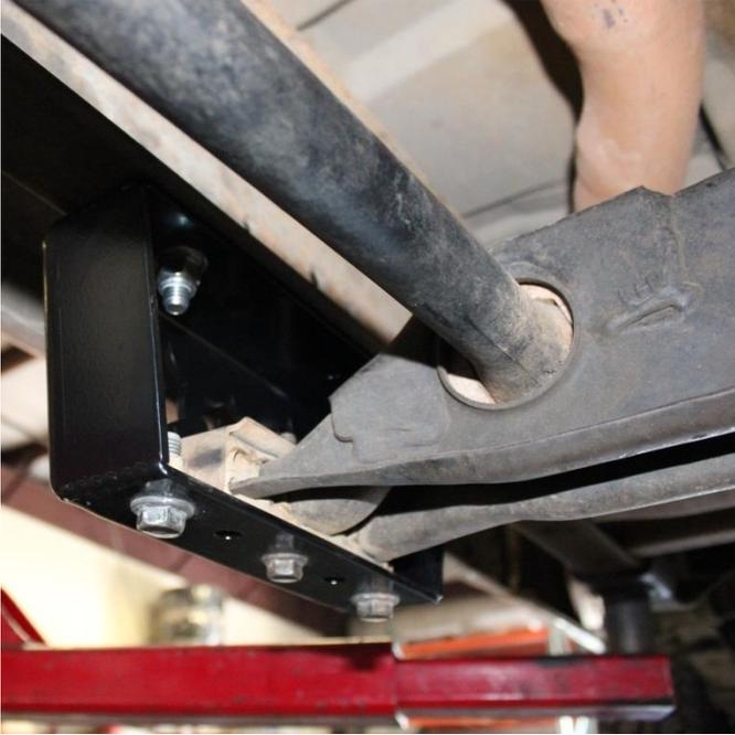
44) install front shock using factory hardware.
