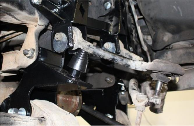
39) Install factory steering knuckle, CV axle and hub assembly as shown below. Tighten to factory specs.
