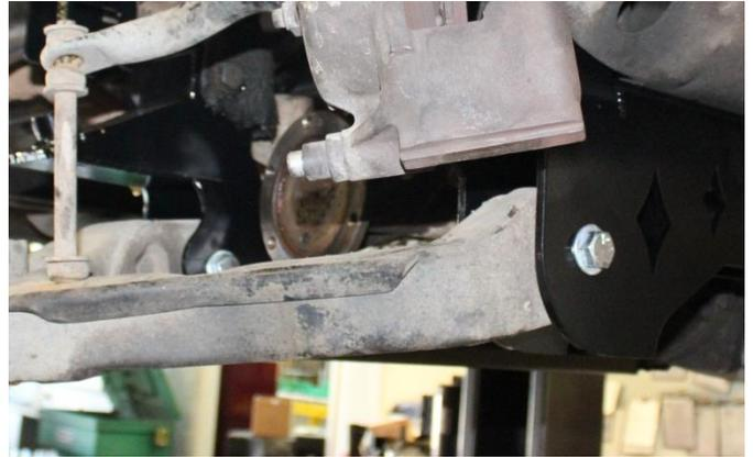
46) Tighten upper alignment cams to 90 ft.-lbs.
