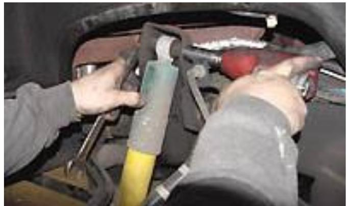
7) Remove The 36mm Axle Nut, Remove the three 14mm hub bolts. Carefully remove hub from knuckle assembly on each side. This will allow removal of the steering knuckle from upper and lower ball joints without fighting the assembly to get the cv axle out first.
