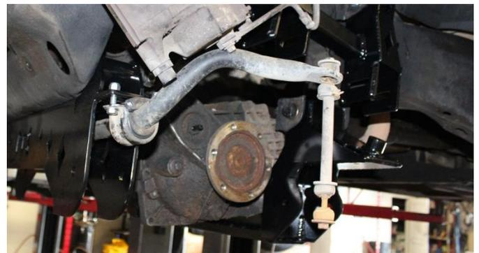
31) Install the lower a arm using the 5/8" x 5" hardware on the front lower and the 5/8" x 6" hardware on the rear. Tighten the hardware attaching the cross member to the frame.
