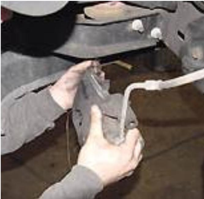
5) Remove nut attaching outer tie rod end to steering knuckle; detach outer tie rod end from steering knuckle using tie rod separator. DO NOT strike threaded area of tie rod end stud. Repeat this process on opposite side of vehicle.
