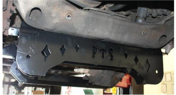
31) Install the factory sway bar using the 3/8" x 1 1/2" hardware.
