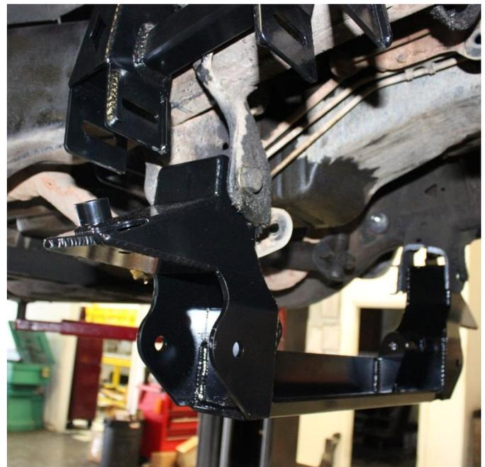
22) Dress Cuts with grinder, making sure that the cut is inboard of the flat area adjacent to the shock mount tower. Clean and spray cut areas with paint or rubberized undercoating.
