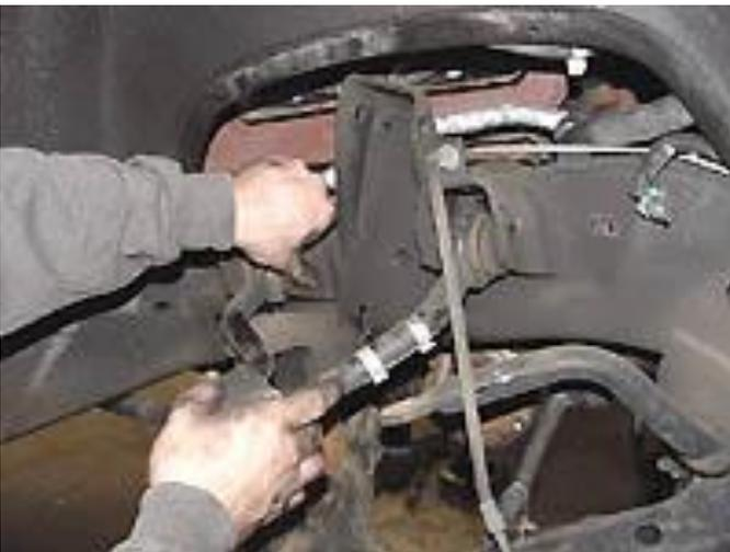
12) Remove the 6 bolts attaching inner end of CV axle to the axle flange, then CAREFULLY remove CV axle assembly. Repeat these steps on opposite side of vehicle.
