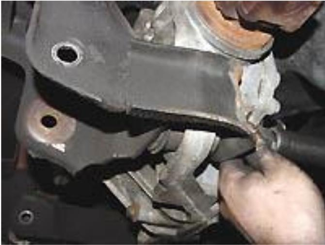
19) Remove torsion bar cross member from vehicle frame as shown. NOTE: 4 door Tahoe's must remove cross member AND outside drop hangers from frame. ALL OTHERS remove cross member by remove the 3 retaining bolts and nuts from the bottom of the frame rail as shown below right.
