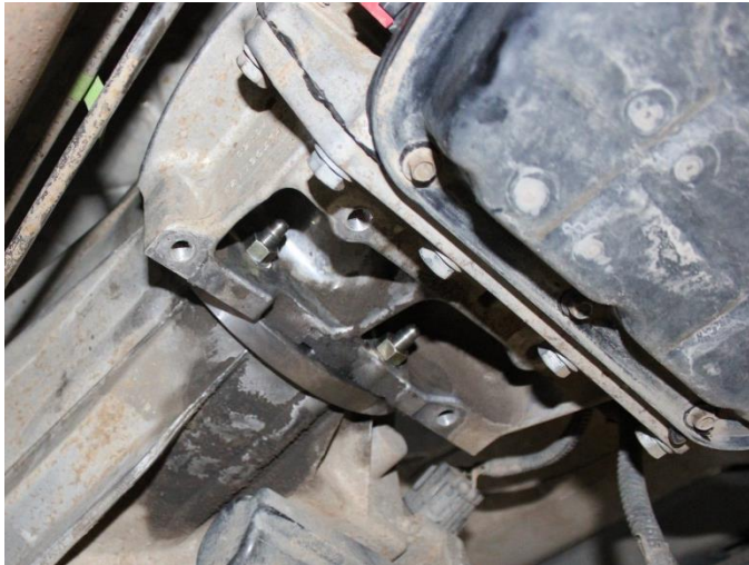
56) Reconnect all electrical plugs on the transfer case.
