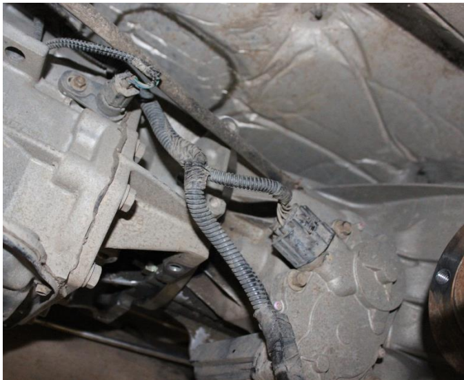
56) Reconnect all electrical plugs on the transfer case.
