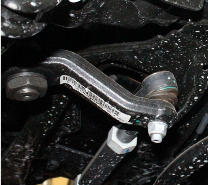
10) Using a hammer, strike the pitman arm to dislodge the tie rod from the pitman arm.
