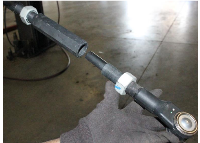
12) Using a die grinder or abrasive saw remove the flat portion of the tie rod.
