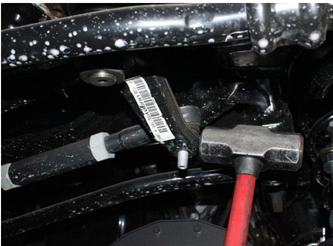
10) Using a hammer, strike the pitman arm to dislodge the tie rod from the pitman arm.
