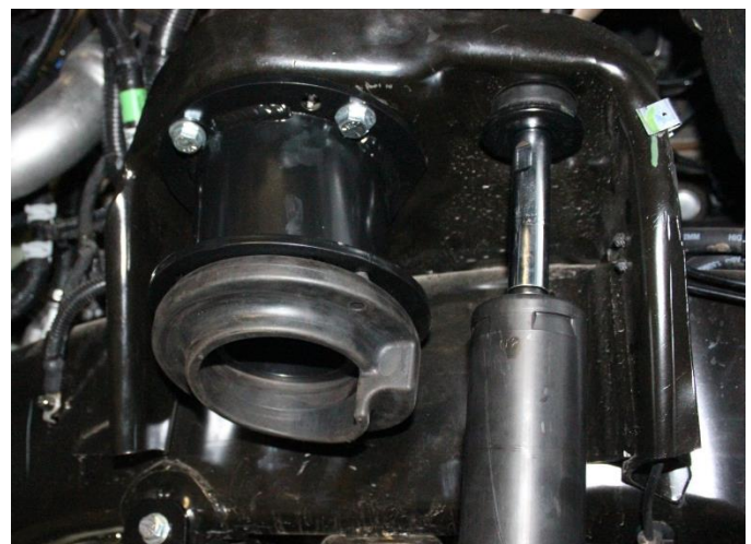
38) Remove the upper shock hardware and lower the axle down enough to install the coil springs. Re-attach the upper shock hardware.
