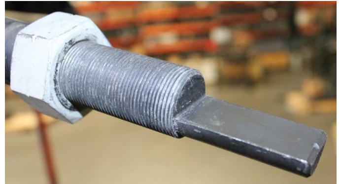
12) Using a die grinder or abrasive saw remove the flat portion of the tie rod.
