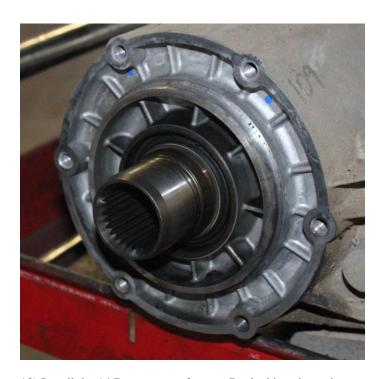
13) Install the 14 Degree transfer case Reclocking ring using the 10mm supplied Allen bolt as shown below. Use Loctite on the threads
