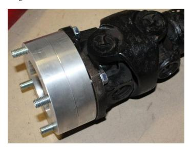
20) Install the front drive shaft to the transfer case. Use Loctite on the treads. DO NOT connect the front drive shaft to the front axle at this time.
