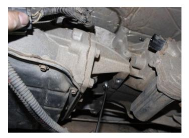
12) Remove the 6 studs on the front side of the transfer case. Using the factory nuts, double nut the stud and to allow the inner nut to back the stud out of the transfer case.
