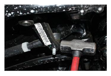
25) Remove the hardware attaching the drag link to the steering knuckle. Save the hardware.
