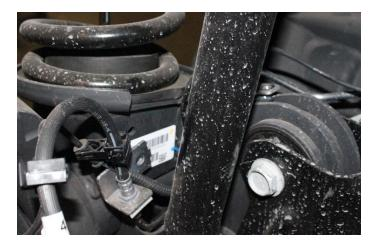
4) Remove the front sway bar end links from the axle mount. Remove the bolts securing the sway bar mounts to the frame and set the sway bar aside, save all sway bar hardware. NOTE the orientation of the sway bar for installation.
