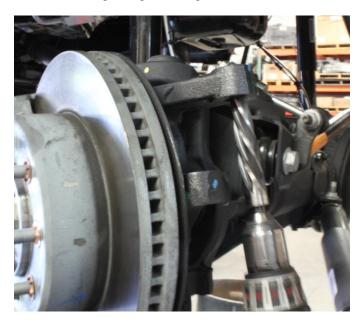
27) Unscrew the tie rod end out of the coupler.
