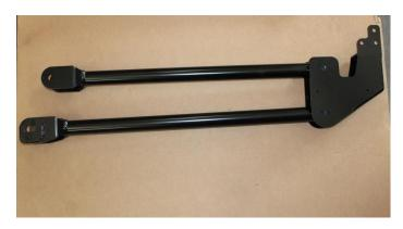
44) Once all nut inserts are installed, re-install the bracket using  $\frac{1}{2}$ " x 1  $\frac{1}{2}$ " hardware. Install the upper link arm using the Factory hardware. DO NOT tighten at this time.
