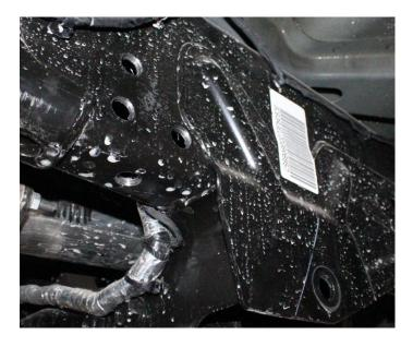
39) With holes enlarged install nut inserts using supplied spacer and tighten bolt till each nut insert crimps itself tight into the frame.
