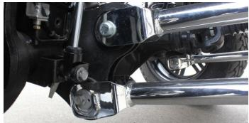
46) Install the track bar bracket as shown, Use the factory hardware threw the factory hole in the frame. Snug the bolt enough to hold the bracket in place. Mark the 3 holes on the bottom side of the frame using the track bar bracket as a guide.
