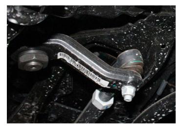
24) Using a hammer, strike the pitman arm to dislodge the tie rod from the pitman arm.
