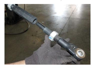
28) Using a die grinder or abrasive saw remove the flat portion of the tie rod.
