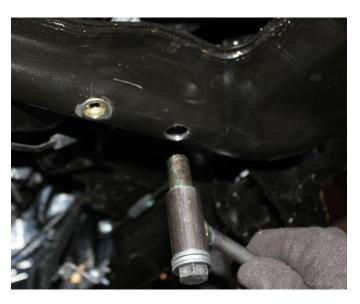
48) Reinstall bracket using the 18mm x 90mm hardware.
