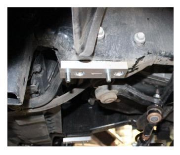
43) Use the 7/16" nuts to attach the sway bar to the drop brackets.
