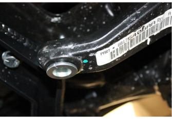
37) Install the sleeve into the steering knuckle as shown below.
