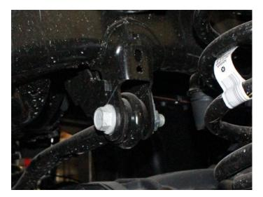
30) Remove the front upper nut and the lower bolts securing the shock to the axle. Save the lower Hardware. Remove shocks.
