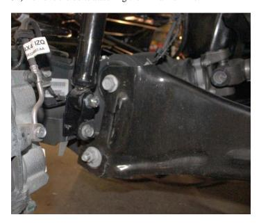
35) Install the FTS 4 Link bracket using the factory hardware.
