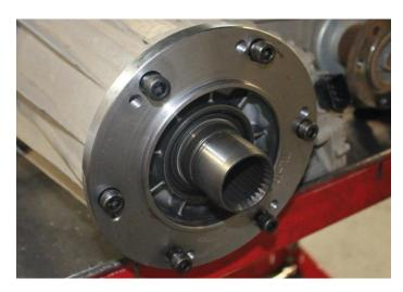
14) Install the supplied 3/8" x 2" studs into the face of the Reclocking ring using the supplied nuts to tighten the studs.
