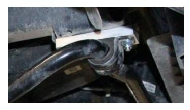
44) Install the bushing and sleeves into the sway bar end links.
