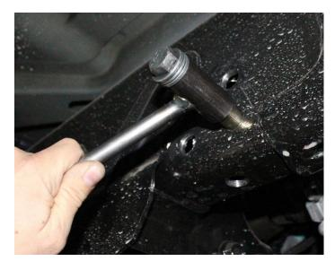
40) Use a 3/8" impact to tighten the nut-serts into the frame as shown.
