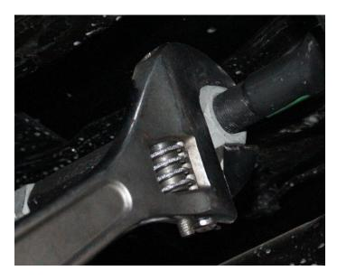
23) Remove the hardware attaching the drag link to the pitman arm. Save the hardware.
