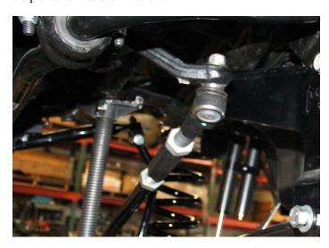
40) Continued. Install washer the factory nut. Use loctie on the threads.
