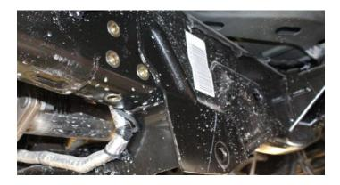
42) Pictured below is upper and lower links Short link is the upper driver side Long lower link is the driver lower
