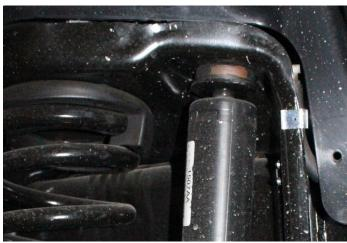
31) Leaving the front axle supported on the 2 jacks raise the truck enough to remove the coil springs. Save the upper rubber insulator, coil springs & shocks for Reassembly. USE EXTREME CARE WHEN WORKING WITH COILS THAT ARE UNDER LOAD!
