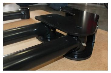
43) Install the bushing and sleeves into the link bars. Prior to installing the bushing Use the supplied grease to lube only the inside hole of the bushing where the steel sleeve rides, DO NOT Grease the outer part of the bushing or the inside of the control arm. Use Bushing # MO2918. Sleeve # DS3642
