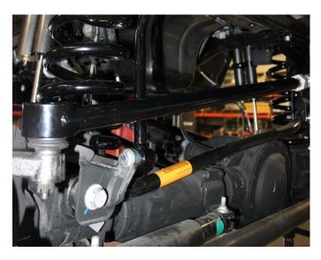
40) Install the other end of the drag link to the bottom side of the pitman arm as shown below.
