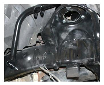
14) Drill the lower hole 1" thru the outside of the frame and  $\frac{1}{2}$ " thru the inside. Install the supplied frame sleeve
