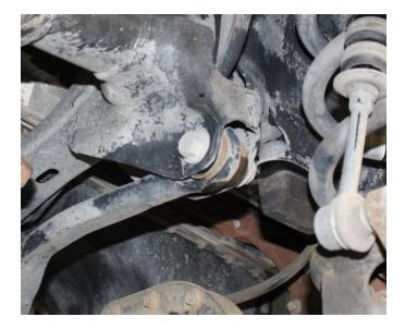
8) Remove the top nuts on the front shocks and the lower bolts securing the shock to the axle. Leave the shock loose inside the factory coil spring at this time. Save the lower Hardware and discard the upper.
