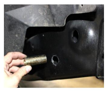
15) After drilling the 1" hole threw the outer portion of the frame insert the sleeve into the frame
