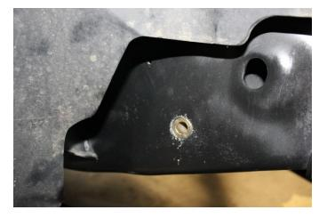
16) Install the shock hoop using the  $\frac{1}{2}$ " x 4  $\frac{1}{2}$ " hardware threw the lower hole and the  $\frac{1}{2}$ " x 1  $\frac{1}{2}$ " threw the upper hole.
