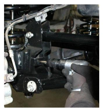
18) Install the lower shock brackets using the factory hardware on the upper hole, Use the 1  $\frac{1}{2}$ " thru the lower back hole. Torque the  $\frac{1}{2}$ " hardware to 70ft.-lbs.
