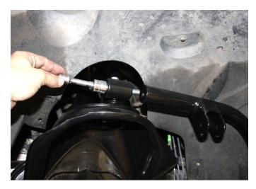
13) With the shock hoop mounted against the frame, Center punch the lower hole.
