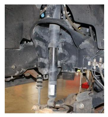
10) Remove the 3 nuts holding the shock tower on, discard the tower , ring and hardware.
