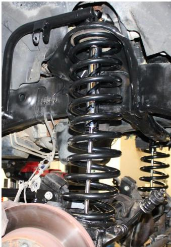
22) Jack up the axle to compress the coil spring enough to get the lower shock bolt in.
