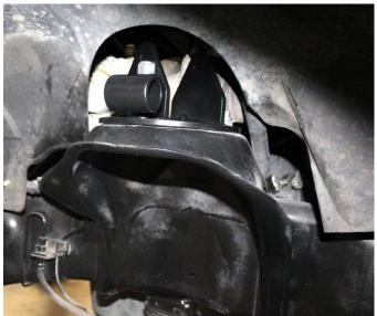
12) Mount the shock hoop to the upper bracket using the  $\frac{1}{2}$ " x 1  $\frac{1}{2}$ " bolt,
