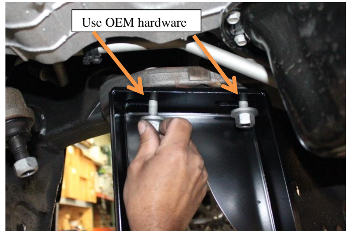
30) Install differential using 1/2" x 2" and 5/8" x 2" on the passenger side and the 1/2" x 3 1/2" on the driver side as shown.
