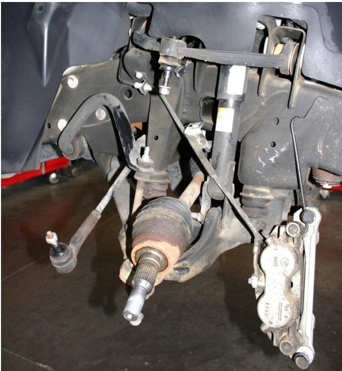
10) Remove the sway bar link ends from the sway bar and lower control arm. Discard links but retain the bushings for reassembly later.
