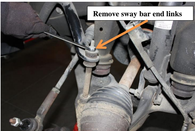
10) Remove the sway bar link ends from the sway bar and lower control arm. Discard links but retain the bushings for reassembly later.
