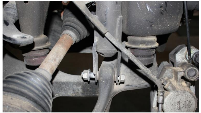
12) Remove the clips attaching wiring harness to torsion bar cross member.
