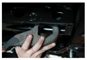
Install supplied 3/8" tall spacer over shock studs
