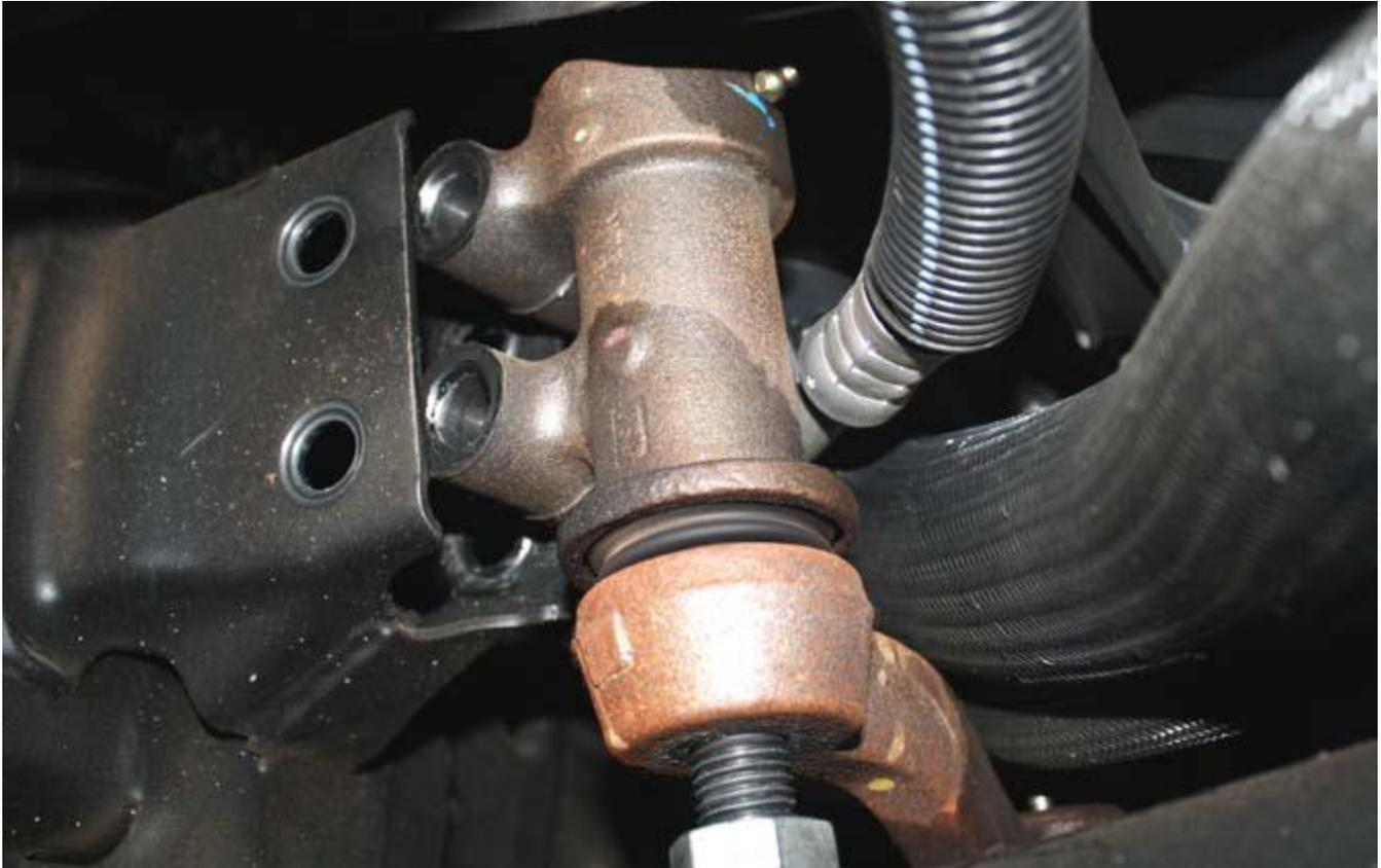
8) There are 2 pitman arm support brackets included in this kit, as of June 20th, 2011. On some of the 2011 and newer GM trucks, there is a new design center link that has a large rubber bushing in the center link where the pitman arm attaches to it. If this vehicle has the new center link, you must use pitman support bracket #3002. If this vehicle has the traditionally designed center link, use the pitman arm support bracket #3001.
