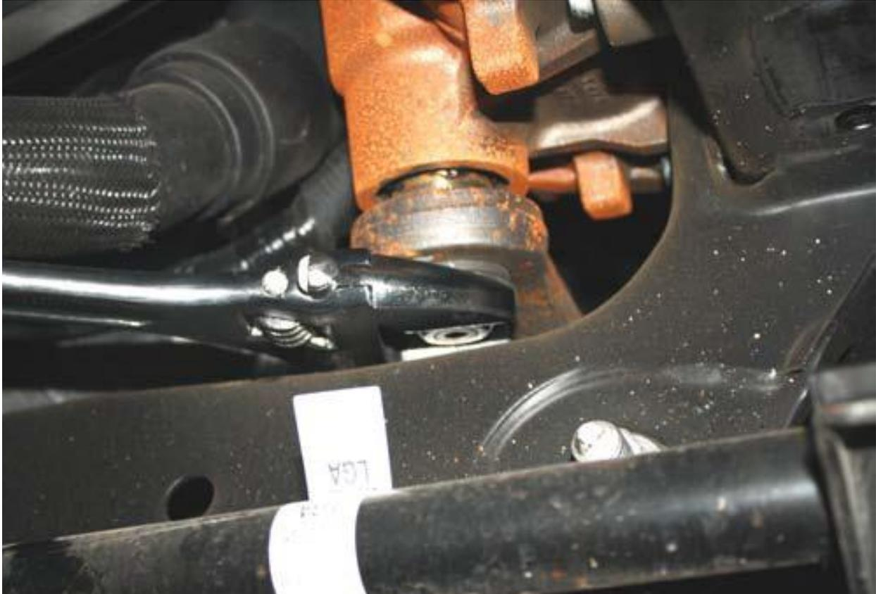
5) Unbolt the steering box from the frame by removing the 3 bolts using a 21mm socket.
