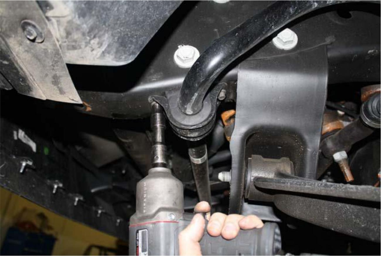
3) Unscrew the factory lock nuts that hold the drag link to the pitman and idler arms, using a 24mm deep socket, and discard them.
