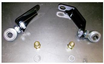
6) Insert one lock washer over each of the drag link studs, and then install the pitman and idler arm brackets on to the pivot ends where hardware was previously removed in steps 3 and 4, at the same time place the rod end which is connected to the Full Throttle Suspension brackets over the drag link studs so that the lock washer is in between the Full Throttle rod end and the drag link.
