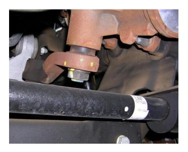
4) Remove the nut holding the idler arm to the idler arm pivot with a 24mm boxed end wrench. On some vehicles, you may have to remove the two bolts (21mm) holding the pivot to the frame brackets in order to get the nut off the stud because of interference with the frame.
