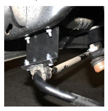
33) Reattach the factory sway bar end links to the axle mounts using the factory hardware. Torque to 40 ft. lbs.
