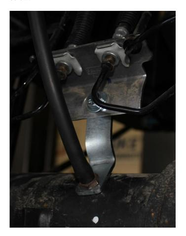
4) Remove the U-bolts from truck and discard. Lower the axle down slowly. Use care not to over extend the brake hose.
