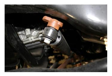
7) Remove the cotter pin and nut from the pitman arm.
