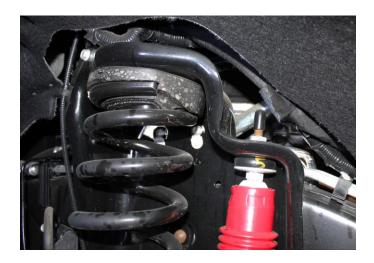
15) Remove the lower shock hardware, Remove shock.
