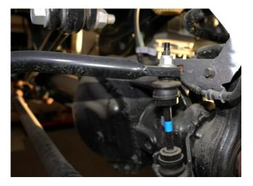
5) Remove the factory sway bar and save hardware for assembly.
