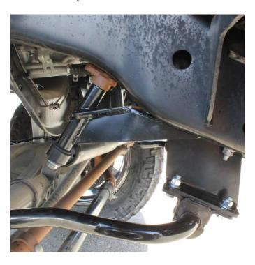
32) Install sway bar frame drop brackets and attach to the frame where the sway bar was originally attached using the factory hardware Using the supplied 7/16" X 1 ½" hardware, attach the sway bar to the new drop brackets and torque to 45 ft. lbs.
