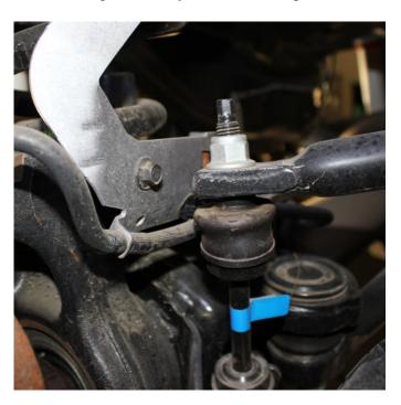
34) Position the factory trac bar into the new trac bar bracket. Note: You may need to raise the axle up or down to align the hole. Using the original bolt insert it from the front side of the bracket towards the back. Torque the trac bar bolt to 400 ft. lbs. See #35 for Instruction on how to install the track bar cam washer
