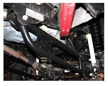
27) Using a floor jack raise the front axle enough to compress the front coils approx. 1". Install supplied front shocks.
