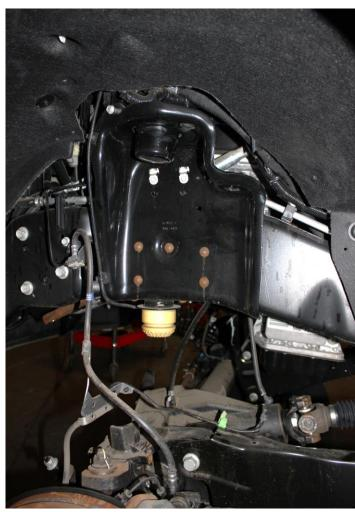
17) Using a die grinder, remove approximately 3/16" from the shock mount as shown below.
