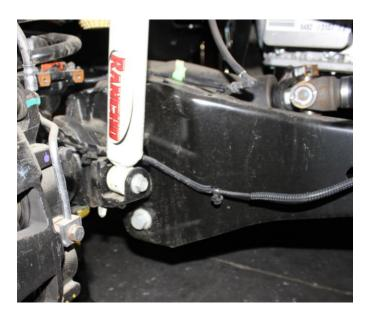
4) Remove the sway bar end links from the axle mount and save with the hardware.
