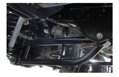
29) Install the new FTS brake lines brackets using the supplied 5/16 x 1" hardware as shown. Reconnect the lower brake line bracket to the factory perch using factory hardware.
