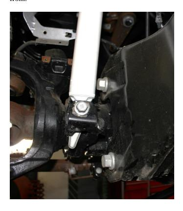
19) With the front axle still supported by the floor jacks remove both front factory radius arms from axle and factory frame mounts. Save the factory frame pivot bolts and the factory front pivot bolt from the axle mounts.
