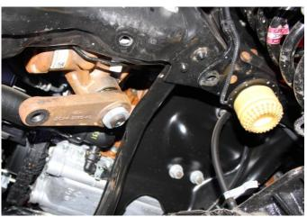
11) Remove the factory pitman arm from the steering box using a large pitman arm puller or large two-jaw puller. Save the hardware and discard the pitman arm.
