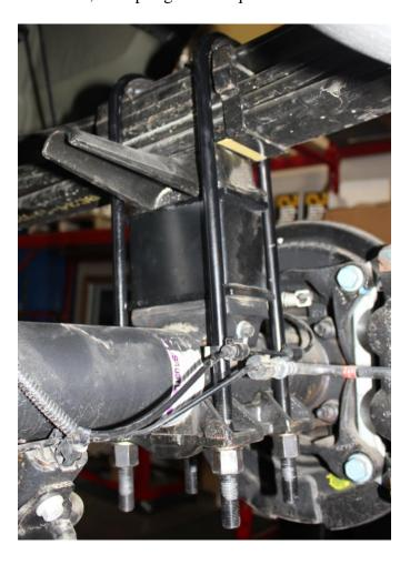
6) Install FTS shock with the factory hardware and torque bolts to 65lbs.
