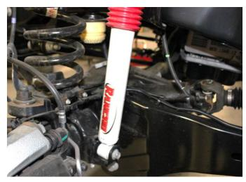
16) Lower the front axle allowing the coil springs to come free of tension. CAUTION WHEN WORKING WITH COIL SPRINGS UNDER LOAD! Remove the coil springs from the truck and discard, save the factory upper coil isolator
