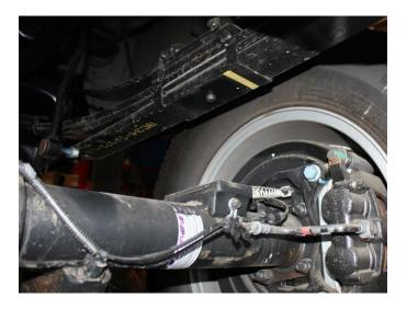
5) Install the rear lift blocks, the factory block will be positioned on top of the new block, with the short center pin of both blocks facing down, to the axle. Using the supplied U-bolts, nuts, washers align axle, lift blocks, and springs and torque to U-Bolts to 90lbs.
