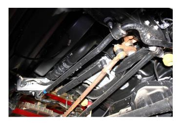
6) Remove the factory steering stabilizer from the frame mount discard hardware. Leave the steering stabilizer connected to the drag link.
