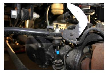
14) Supporting the front axle with two floor jacks, Remove the upper shock mounting hardware.
