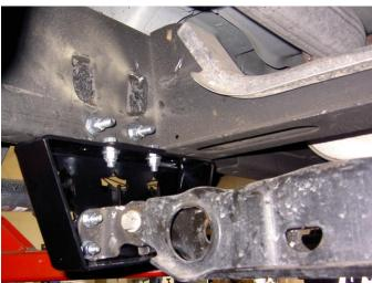
60) Mount the torsion bar drops with the  $7/16 \times 1\frac{1}{4}$  bolts and hardware supplied, DO NOT tighten at this time
