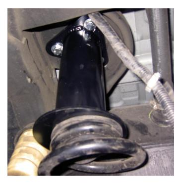
6) Install upper and lower trailing arm drop brackets as show
