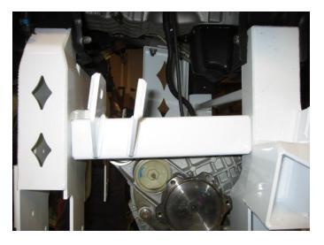
24) Install the upper a arm drop bracket to the rear cross member using the 5/8 x 6" bolts and hardware.
