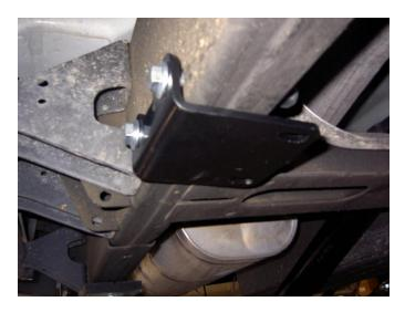
59) Drill the previous marked holes with ½" drill bit, BECAREFULL not to drill into the hard line on the frame
