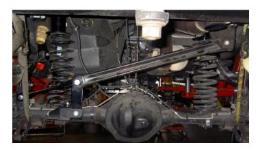
8) Place a floor jack under the rear axle. Set the upper coil insulator on top of the coil spring and position the top of the coil into the frame pocket. Push the bottom of the coil spring onto the axle pad and raise the floor jack under the axle to hold the coil spring in position. Repeat this with the opposite coil spring.
