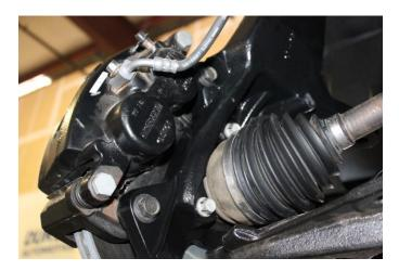
18) Locate T538 outer tie rods. Loosen the jam nut and remove the factory outer tie rods and discard, leaving the factory jam nut on the inner tie rod. Install the new outer tie rod onto the inner tie rod until it makes contact with the jam nut. Attach new tie rod end to the knuckle with the supplied nut and torque to 45 lbs.
