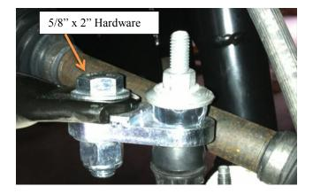
23) Locate 8511 Brake Line Bracket and 5/16"x 1" hardware. Position the new bracket into the factory brake line bracket location and attach with the factory hardware and the 5/16" hardware. Attach the factory brake line bracket to the new bracket. **Carefully** bend the hard brake line and attach with the supplied 5/16" hardware. Torque to 15 ft.-lbs. As shown in picture below.
