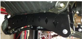
20) Locate 8504L Driver, 8504R Pass Sway Bar Frame Bracket, and four 10mm stock CV axle bolts with supplies washers. Position the frame bracket on the frame so that sway bar will be farther back from the suspension and attach with the 10mm hardware.
