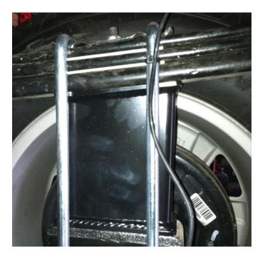
12) On the passenger side, locate the original line clamp Hole in the top of the frame and measure 2" down the inside of the frame and drill a <sup>1</sup>/4". Insert the previously removed upper ABS line clamp into the new hole on the inside of the frame. Re-insert the lower ABS line clamp back into the stock location. Use zip ties and attach the ABS line to the U-Bolt. Keep the line taught at the block and ensure that there is enough slack in the line for full travel of the rear axle.
