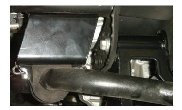
22) Locate 8507 Sway Bar Extension Mounts and the supplied 5/8"x2" hardware. Position the Sway Bar Mount so that it is on the bottom of the sway bar with the SHORTER side of the mount against the stop plate end of the mount. Attach with the 5/8 hardware and torque to 135 ft.- lbs. Locate the factory sway bar end links and attach to the new mount and the lower control arm. As shown in picture below.
