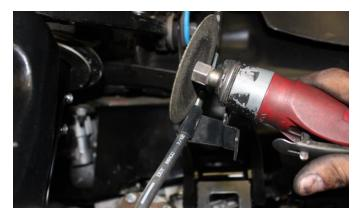
11) Remove the bolts connection the strut to the lower control arm. Retain hardware for reinstallation.
