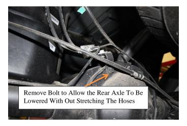
3) Remove the ABS line clip from the top of the frame and at the axle.
