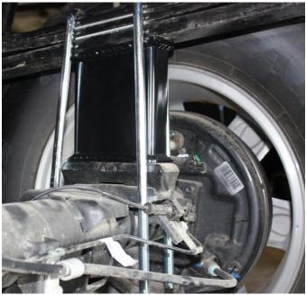
The Short Side Of The Block To The Front And The Tall Portion To The Rear Of The Truck
