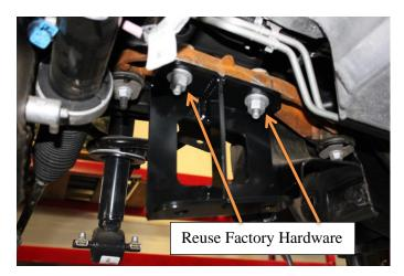
2) Locate 8502 Driver side Differential brackets and the factory diff hardware. Install the brackets to the factory mounts with the taller part of the brackets to the front of the truck with the factory hardware.
