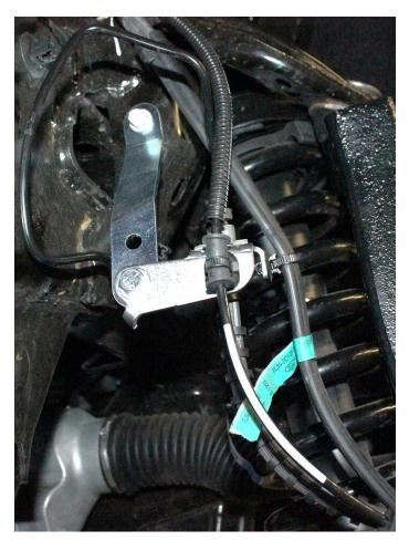
52) Mount factory brake line bracket to the side of the knuckle using the factory hardware.
