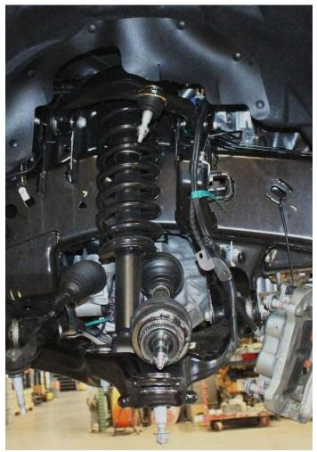
17) Remove the lower strut mount nuts. Save the hardware.
