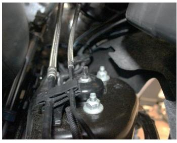
19) Remove the front and rear lower control arm bolts from the frame pivots point and remove the lower control arm from the truck. Save hardware and lower control arm.
