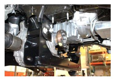
34) Push the driver rear differential bolt all the way thru the bushing and cross member as shown below. Using the supplied 14mm Nylock nut and washer.
