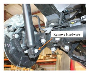
5) Supporting the rear differential, remove the U-bolts, lower axle down, remove factory block. Use care not to over extend the brake hose.
