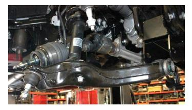
40) Install the lower control arms into the cross members using 18mm x 150mm bolts. Leave hardware loose. Torque lowers A arms bolts to 180 ft.-lbs.
