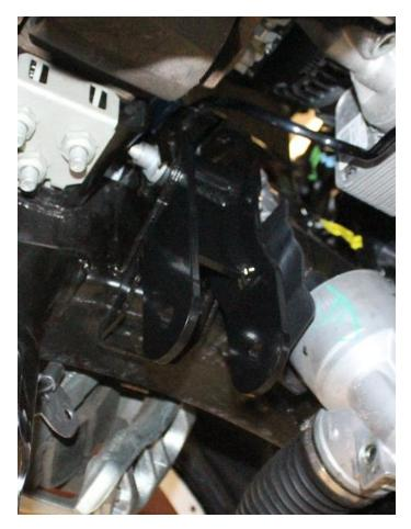
29) Install the passenger side differential drop bracket using the supplied 9/16° x 4  $\frac{1}{2}$ ° hardware onto the differential as shown below.
