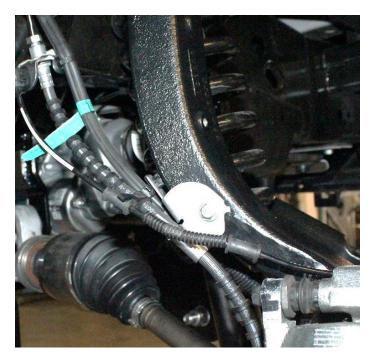
53) Install the FTS driver and passenger sway bar drop brackets so the sway bar is pushed towards the FRONT of the vehicle using the factory hardware as shown below.
