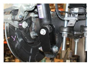
8) Install the E Brake bracket using the 5/16" x 1" hardware as shown below.
