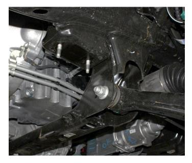
7) Remove the front drive shaft bolts where they attach to the front differential. Discard hardware.
