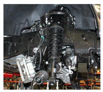
39) Connect the lower strut mount to the factory control arm as shown below using the factory hardware.
