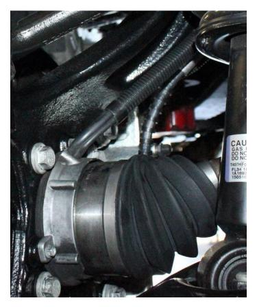
50) Reattach the factory tie rod to the steering knuckle using the factory hardware.
