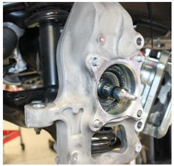
16) Loosen the upper and lower ball joint nuts. Disconnect the upper and lower ball joints from the steering knuckle by striking the knuckle with a large hammer next to each ball joint on the knuckle to dislodge the ball joints. Use care not to hit the ball joints when removing. Retain hardware and remove the knuckle and actuator. Use extra care not to over extend the C.V. axle shaft when removing the knuckle.
