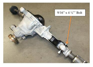
30) Cut the rear diff bolt down to  $3\frac{3}{4}$  as shown below.
