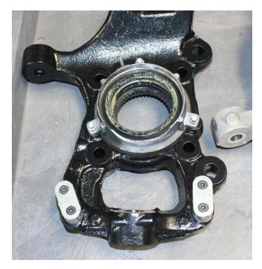
43) Install the spindle onto the upper and lower control arms. Torque the upper ball joint to 85 ft.-lbs. and the lower ball joint to 110 ft.-lbs.
