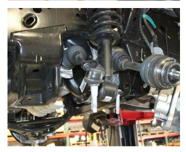
20) Remove the strut assembly from the vehicle and mark "Driver" for assembly to install later with upper strut spacer.
