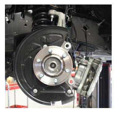
12) Disconnect the ABS wire from under the fender well.
