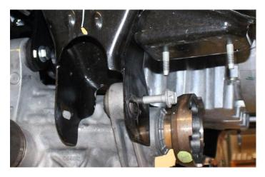
33) Install the passenger side differential support as shown below using the factory hardware.
