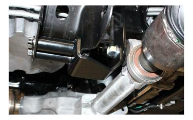
33) Install the FTS rear cross member in the factory rear lower control arm pockets. With the open portion to the front of the vehicle. Mount the cross member using the factory control arm pivot hardware. Leave all hardware loose at this time.
