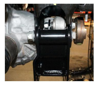
35) Install the FTS front cross member into the factory front control arm pockets using the factory hardware. Leave the hardware loose at this time.
