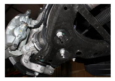
6) Remove the sway bar frame mounts from the frame, Remove the sway bar. Save the hardware and sway bar.
