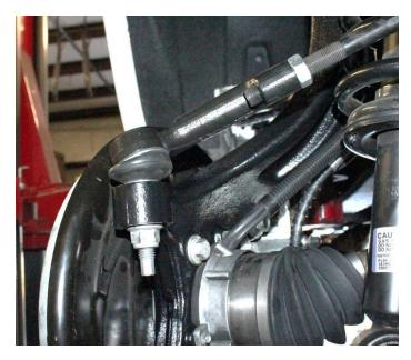
51) Install the front brake line bracket using the factory hardware at the top and the 5/16° x 1° hardware at the bottom. After installing the factory brake line bracket, check to insure full movement by steering the knuckle back and forth, and make sure none of the ABS lines, brake lines, or vacuum lines are interfering during full test Movement of the knuckle.
