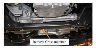
23) Remove the driver side rear differential mount hardware.
