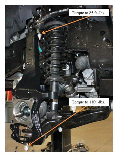
44) Install the factory hub. Torque the four 14mm bolts to160 ft.- lbs. Install the ABS wheel speed sensor. Make sure the end of the sensor is clean. Apply Loctite to the threads.
