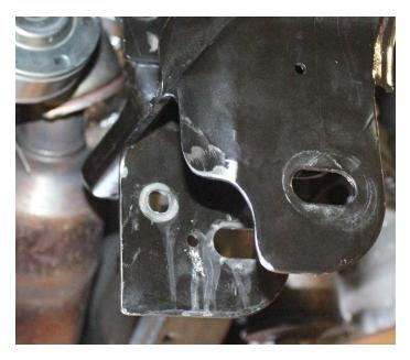
28) Install the driver upper differential mount. The upper differential mounts will be placed into the factory upper differential mounts using the factory upper differential mount hardware. Leave the hardware loose in preparation for the differential installation.
