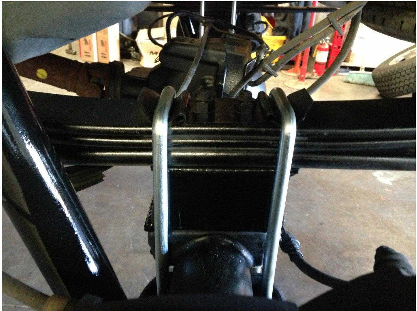
Install Rear Lift Block As Show In Picture Above
