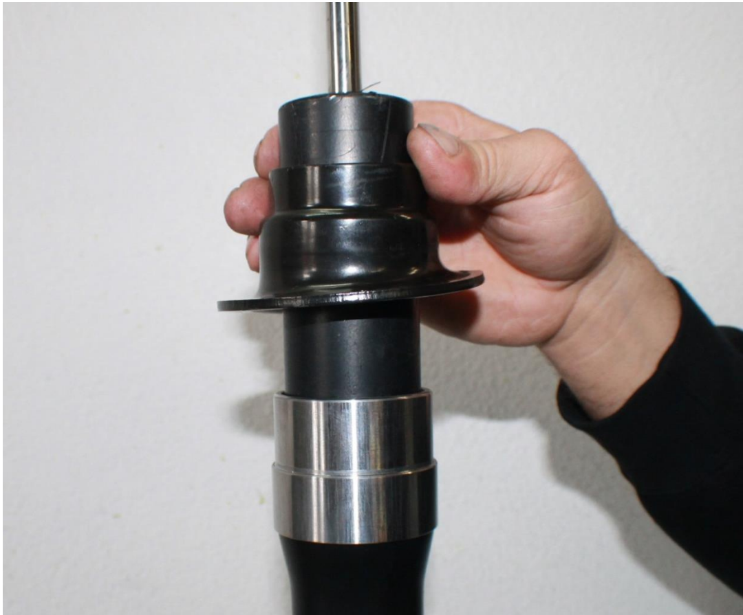
Installation Picture Of Spacer Installed
