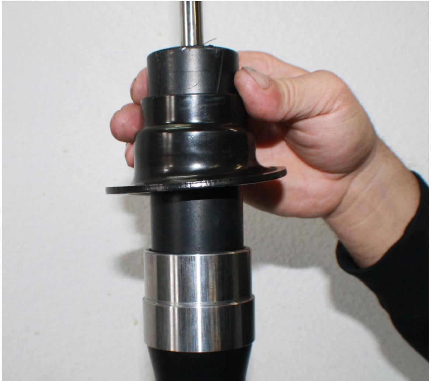
Installation Picture Of Spacer Installed
