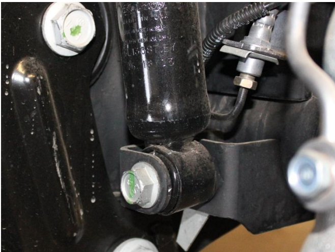
14) Remove the front upper nut and the lower bolts securing the shock to the axle. Save the lower Hardware. Remove shocks.
