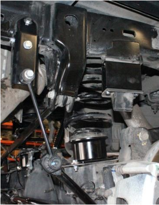
24) Install rear brake line bracket as shown.
