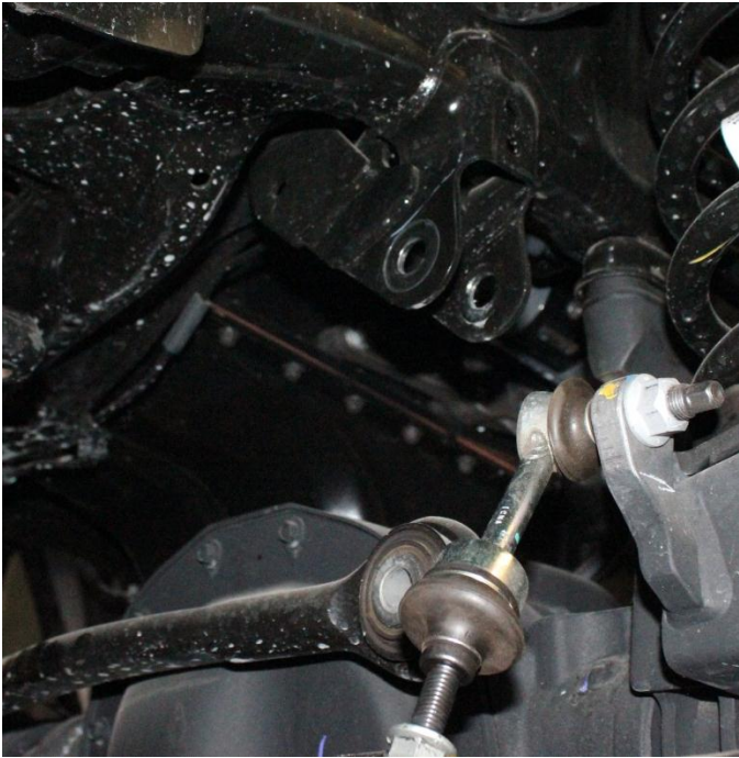
14) Remove the front upper nut and the lower bolts securing the shock to the axle. Save the lower Hardware. Remove shocks.
