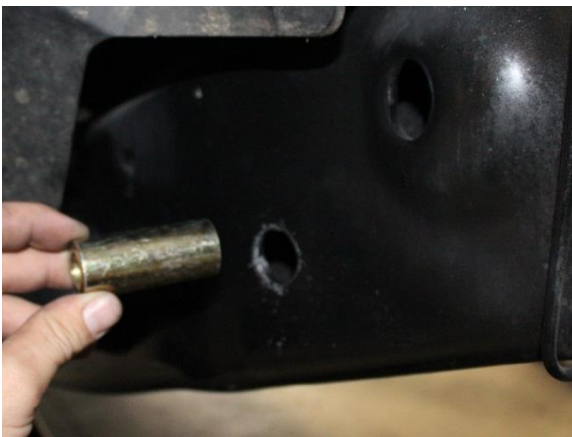
31) Drill the lower hole 1 " thru the outside of the frame and \frac{1}{2} " thru the inside. Install the supplied frame sleeve
