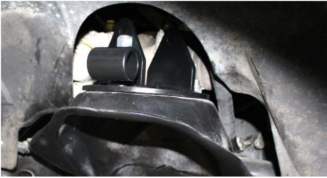
29) Mount the shock hoop to the upper bracket using the \frac{1}{2} " x 1\frac{1}{2} " bolt,
