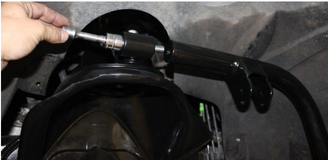
30) With the shock hoop mounted against the frame, Center punch the lower hole.
