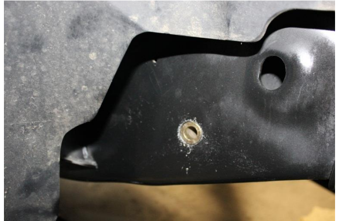
33) Install the shock hoop using the \frac{1}{2} " x 4\frac{1}{2} " hardware thru the lower hole and the \frac{1}{2} " x 1\frac{1}{2} " thru the upper hole.
