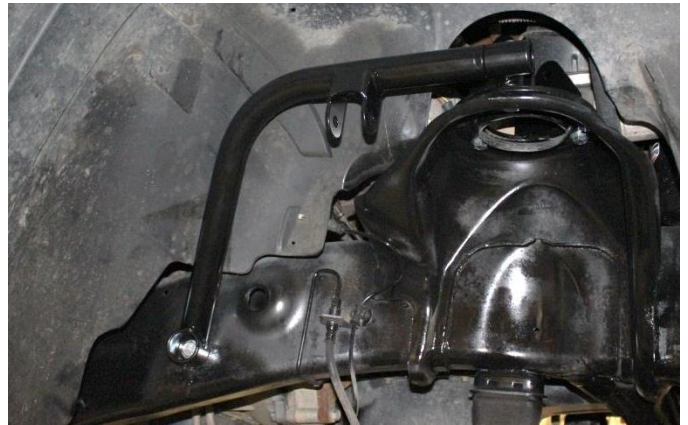
34) Drill out the rear hole to \frac{1}{2} " or slightly larger.
