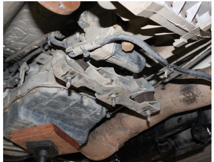
58) Reinstall the factory transmission cross member.
