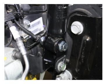
6) Reinstall the brake line bracket to the lower coil perch using factory hardware. Torque to 20 ft.-lbs.
