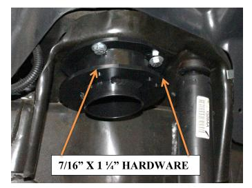
3) Reinstall Front coil springs into coil pocket; make sure you don't forget the rubber isolator on the top of the coil spring
