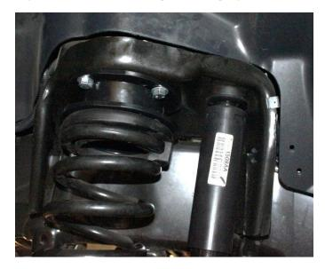
4) Install the FTS lower shock extension using the factory bolts and hardware. Torque to 95 ft.-lbs.
