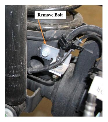
5) Remove the track bar bolt from the frame. Retain hardware for Reinstallation.
