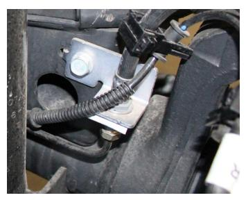
8) Reconnect factory swat bar using factory hardware.
