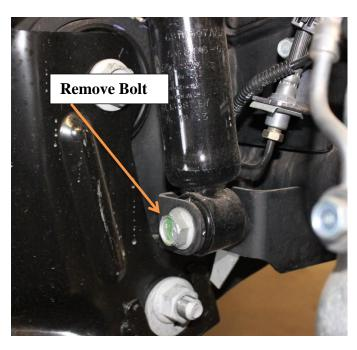
7) Remove coil spring from the truck by lowering the axle down, carefully not to over extend the ABS or Brake lines.
