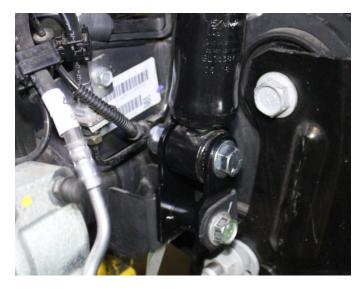
5) Raise the floor jack until the spring is in the proper compressed. Install the shock into the shock extension using the  $9/16 \ge 3 \frac{1}{2}$ " bolts and hardware. Torque to 95 ft.-lbs.
