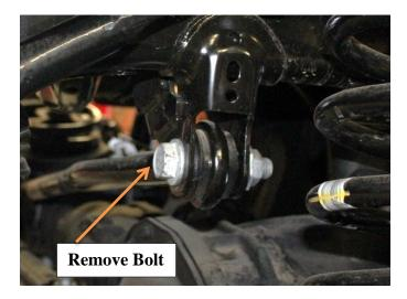
6) Front lower shock bolt. Retain hardware for Reinstallation.
