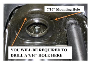
2) Using the supplied 7/16" x 1  $\frac{1}{4}$ " bolt and washer, Install the bolt thru the coil spacer then thru the frame
