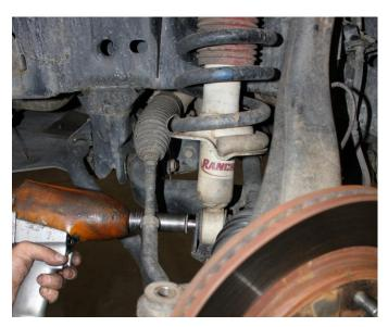
17) Reconnect upper ball joint. Insert new cotter pin
