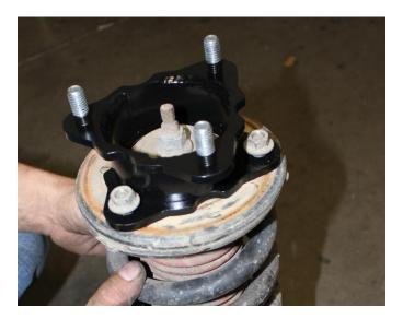
14) Strut assembly will be rotated 180 degrees for re-installation.
