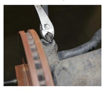
7) Loosen upper ball joint nut.
