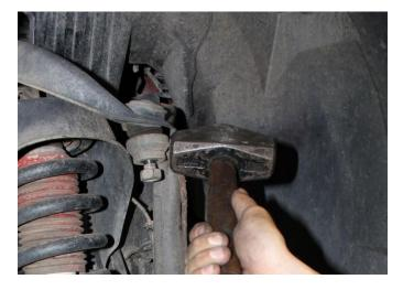
11) Remove lower strut mounting bolt/nut
