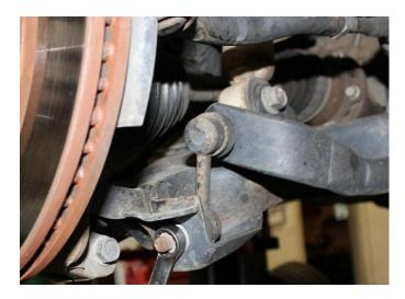
4) Remove three upper strut mounting nuts.
