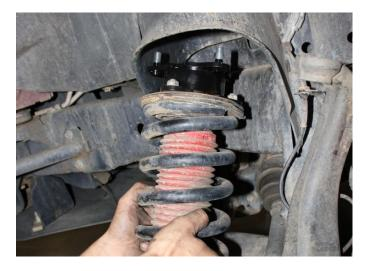
15) Reattach in vehicle with provided hardware and tighten.
