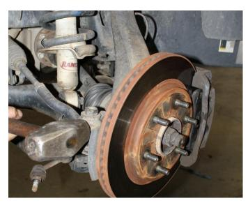
10) Strike the steering knuckle to dislodge the upper ball joint. Remove ball joint from knuckle.
