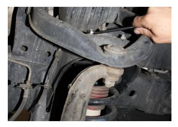
16) Reconnect lower strut bolt and tighten to 120ft.lbs.
