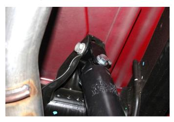
10) Install the shock into the lower mount using the factory hardware Tighten to 120 lb.-ft.
