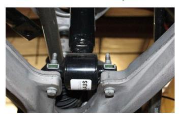
13) Remove the strut from the vehicle. Repeat on opposite side
