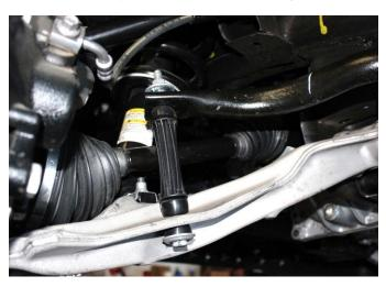
37) Install the brake line support bracket onto upper control arm using the ¼" nuts and washers provided. Tighten to 7 lb.-ft.
