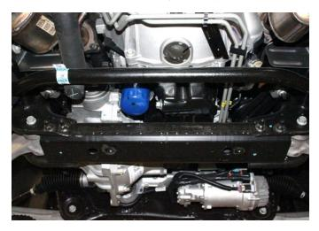
22) Re-install the front drives haft using the factory hardware and clamps. Tighten to 30 ft-lb.
