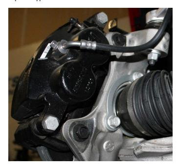
8) Remove the sway bar end link bolt using a 15mm socket and a 15mm open end wrench. Repeat on opposite side
