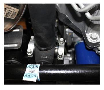
23) Mark the position of the alignment cams. Remove the  $21\mathrm{mm}$  UCA nuts, cams, and bolts.
