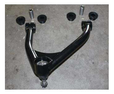
26) Install the FTS upper control arm. The upper ball joint will be angled towards the rear of the vehicle. Install the cam bolts and cams. Line up your markings
