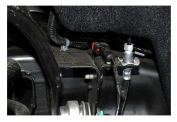
4) Unclip the ABS line at the upper control arm.
