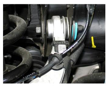
5) Unbolt the brake line retention bracket on both sides.
