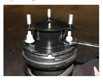
28) Re-install the strut into its stock location. Loosely install the 7/16 nuts on the upper mount.
