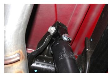
9) Install the shock extension into the upper mount using the factory bolt. Do not tighten.
