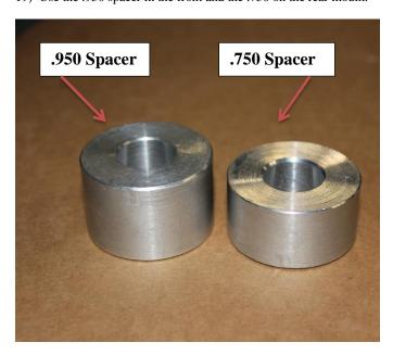
20) Using the supplied  $12 \text{mm} \times 1.75 \times 120 \text{mm}$ , Install the tall differential drop spacer between the frame and the factory differential mount to lower the front down. Install the shorter spacer to the rear allowing the differential to be tilted upwards in the rear.
