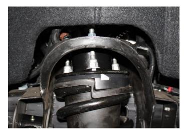
29) Using a cutoff wheel, trim 1/2" off the end of the lower strut bolts
