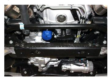
17) Support the front differential and remove rear cross member.
