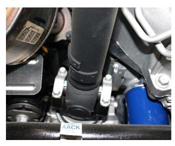
15) Disconnect the front drive shaft front the differential, Don't Remove the drive shaft. Slide the driveshaft back off the yoke.
