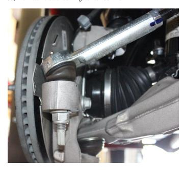
34) Install the front brake calipers using the factory hardware and 18 mm socket. Tighten to 146 ft-lbs.
