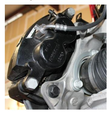
35) Reconnect the inner CV shaft using the factory hardware. Tighten to 45 ft-lb.
