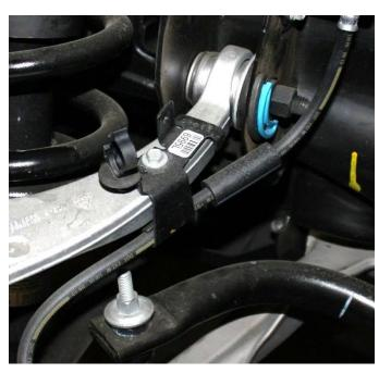
6) Unbolt the tie rod end using a 21 mm socket. An additional wrench may be needed to keep the ball joint from spinning. Strike the knuckle as shown . Repeat on opposite side
