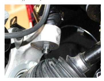
33) Re-install the tie rod. Tighten to 100 ft-lb
