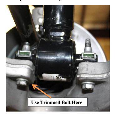
31) Tighten the three upper strut mounting nuts to 45 ft-lb.
