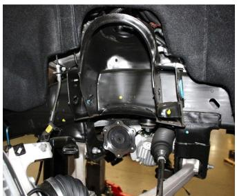
25) Install the bushing and grease fittings into the control arm as shown.
