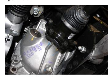
36) Reinstall the sway bar end links on both sides. Tighten to 45 lb-ft.
