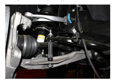
9) Separate the upper ball joint from the steering knuckle. Repeat on opposite side.
