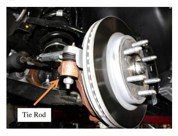
7) Separate the upper ball joint from the steering knuckle. Repeat on opposite side.
